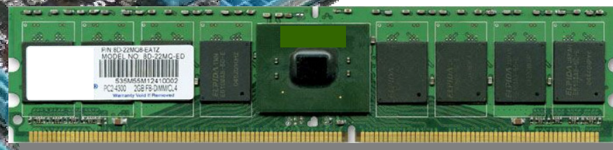
DRAM (WB-BGA) DRAM Module (PCB)
